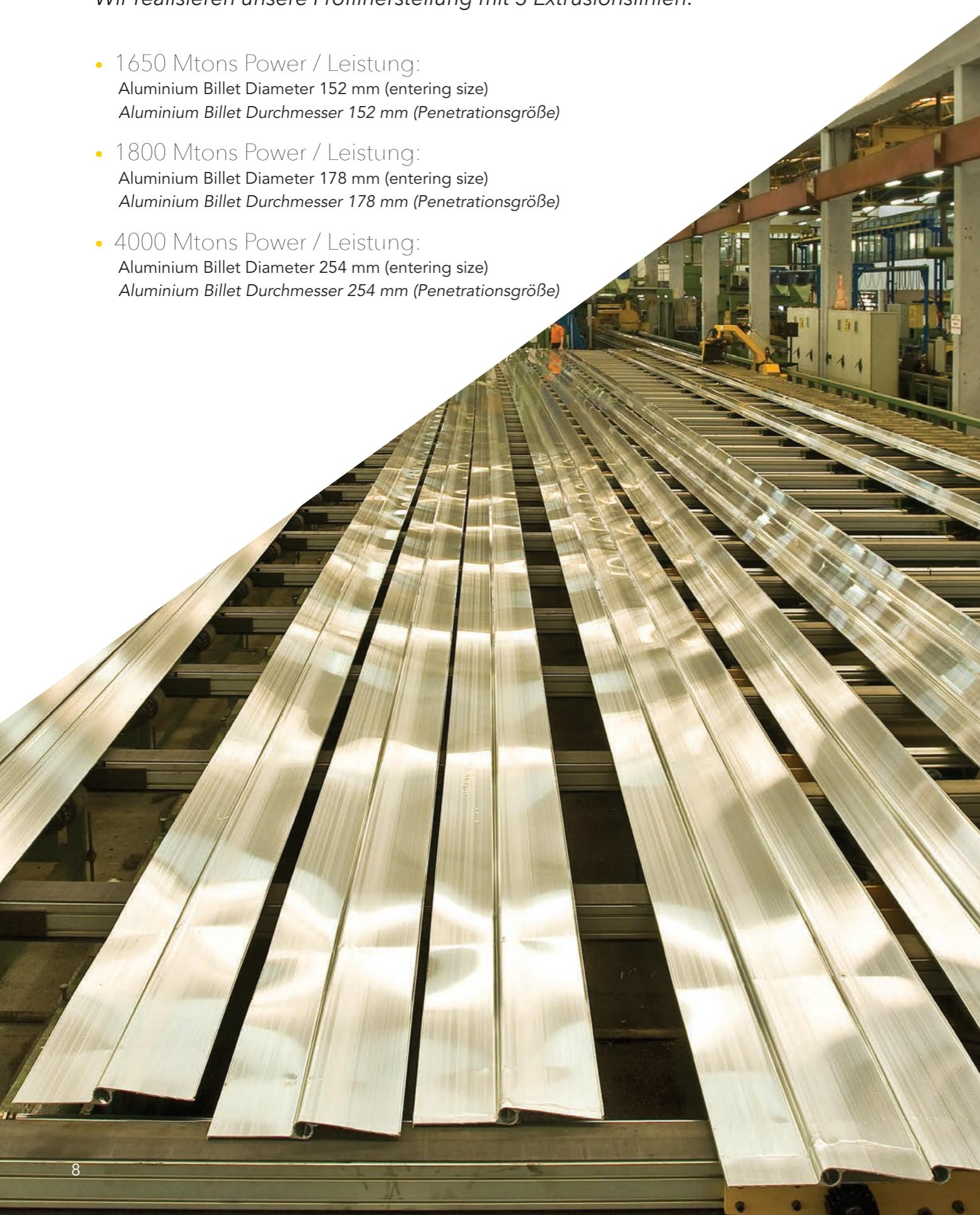
Çuhadaroğlu has an annual production capacity of 20.000 tons extruded aluminium sections through 1650-Mtons, 1800-Mtons and 4000-Mtons aluminium extrusion presses.
